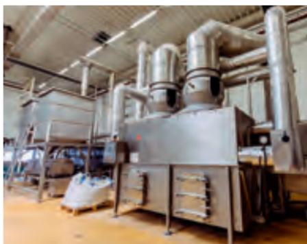
**The roaster forms the company’s core. After roasting a certain type of nut or seed, the oven is thoroughly cleaned.**
